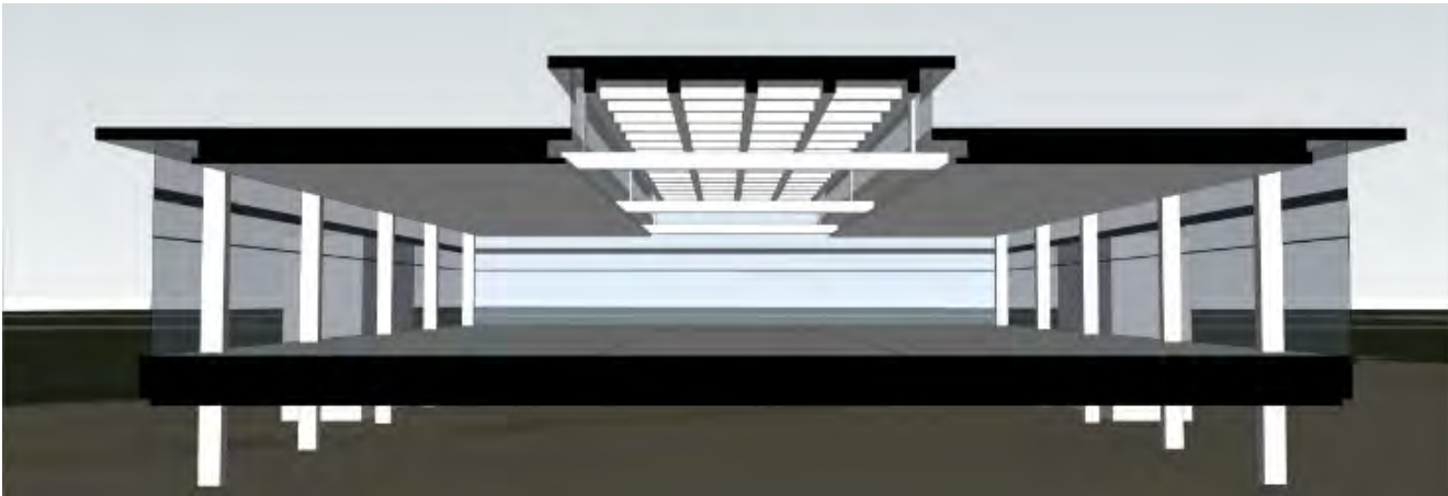
CONCEPTUAL SECTION OPTION 1: CENTRAL CLERESTORY
